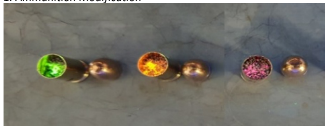
Figure 1. NTA ammunition modified with yellow, orange, and red dyes.
